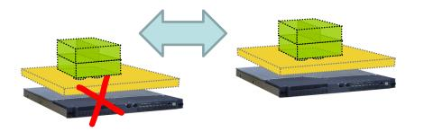
Hardware Fault Tolerance with deterministic replay or checkpointing
